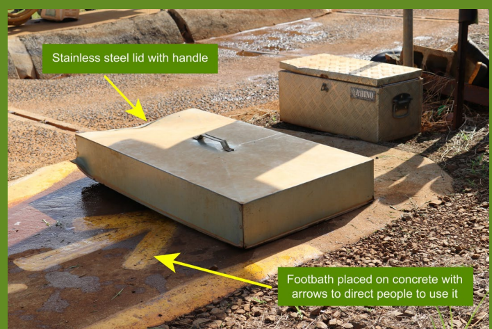
Footbath located on hard paved surface
